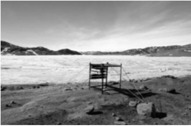
Fig. 2 Sunlight exposure experiment of collagen artificial skins at the Kizahashi raised beach in Skarvsnes of Luetzow-Holm Bay region in mid-summer.
